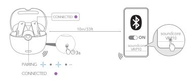
Open the charging case, then press and hold the button on the charging case for 3 seconds to enter Bluetooth pairing mode. Select "soundcore VR P10" from your device's Bluetooth menu to connect.
