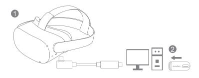
You need a charger that supports USB PD (Power Delivery) and has a minimum output of 9V/2A, otherwise this function might not work properly.
